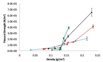
FIGURE 2. Flexural strengths of silica, polycyanoacrylate-modified, 5 mol % aminated silica and polycyanoacrylate-modified, 0.25 mol % aminated silica aerogels: strength of various density silica aerogels  $(0.035-0.215 \text{ g/cm}^3)$  (blue diamond line); strength of CVD-treated silica aerogels (red square line); CVD-treated, 5 mol % aminated silica aerogels (green circle line); CVD-treated, 0.25 mol % aminated silica aerogels (black triangle line).
